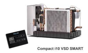
The compressor continuously changes its running speed depending from ambient and set temperature. The compressor operates at maximum power to cool rapidly the cabins, but reaching the set temperature, it reduces the power and electric consumption. In this way it maintains the optimal comfort level with the minimum consumption. The inverter works between 20 and 100 Hz.
