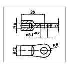
TYPE 1 Welded Eyelet
