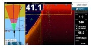
Heading Line View integrates ForwardScan depth data with the heading line on the navigation page of your Simrad<sup>®</sup> display, with simple colour-coding to represent deep, medium and shallow water.
