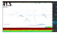
Individual mid water fish. Amazing detection of a jig shown as it drops from 10m to the bottom at 41m.
