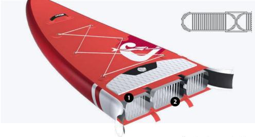
**CREMINISTRAT Double Chamber** PLF Double air chamber core made of pre-laminated (1) composite material without gluing, for a board with exceptional performance in terms of stiffness/weight ratio and stability. The central chamber (2) with dedicated valve ensures improved performance plus greater safety during use in the event of air leaks caused by accidental punctures.
