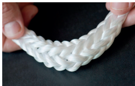
Single braid Dyneema® without HPS treatment: the braid is soft and "airy".
