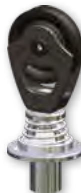
Item Code 5400715 BLOCK SCREWED Weight = 0.75kg 4x Ø6mm screws SWL = 1300kg
