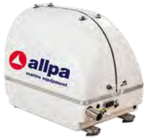
Paguro 3 SY Item Code G03103 Continuous electric power DIN @ 50Hz 3kVA – 3.0kW Weight (incl. soundproof hood): 90kg Dims. 636x433x547mm (lxwxh)
