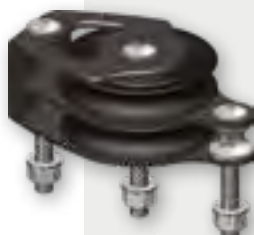
Item Code 5400712 Double Foot Weight = 0.26kg 3 x Ø8mm screws SWL = 1300kg
