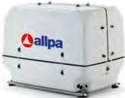
Paguro 5.5 SY Item Code G05105 Paguro 6000 Item Code G06100 Continuous electric power DIN @ 50Hz 5.0kVA - 4.5kW / 6kVA – 5kW Weight (incl. soundproof hood) = 110 kg / 130kg Dims. 660x460x595mm / 684x486x595mm (lxwxh)
