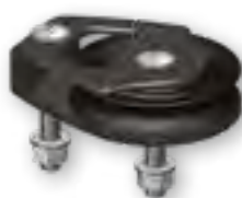
Item Code 5400711 Foot Block Weight = 0.16kg 2 x Ø8mm screws SWL = 1300kg
