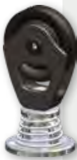
Item Code 5400614 BLOCK PAD-EYE Weight = 0.26kg 4x Ø6mm screws SWL = 800kg
