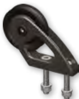
Item Code 5400716 Vertical Fix Weight = 0.18kg 2 x Ø8mm screws SWL = 1300kg
