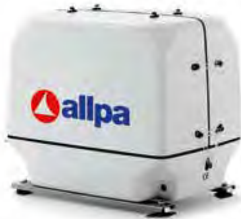
Paguro 12000 V Item Code G12100/V Continuous electric power DIN @ 50Hz 12kVA – 10kW Weight (incl. soundproof hood): 165kg + 15kg (Inverter) Dims. 794x487x615mm (lxwxh) Generator Dims. 250x220x330mm (lxwxh) Inverter
