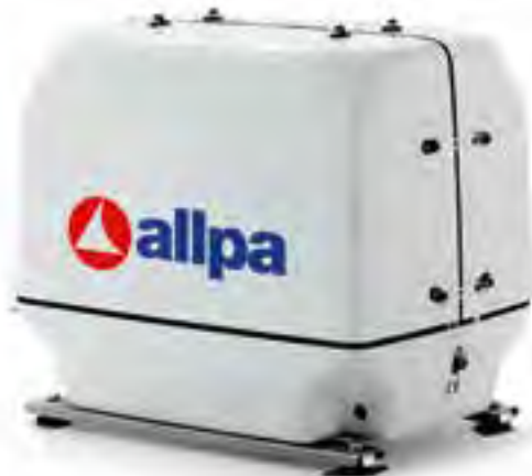
Paguro 6500 Item Code G06115 Continuous electric power DIN @ 50Hz 50Hz 6.5kVA – 6kW Weight (incl. soundproof hood): 170kg Dims. 794x487x615mm (lxwxh)
