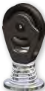
Item Code 5400714 BLOCK PAD-EYE Weight = 0.41kg 4x Ø8mm screws SWL = 1300kg
