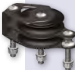
Item Code 5400712 Double Foot Weight = 0.26kg 3 x Ø8mm screws SWL = 1300kg
