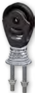
Item Code 5400713 BLOCK U-BOLT Weight = 0.32kg 2x Ø8mm screws SWL = 1300kg
