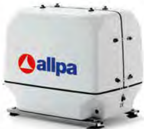
Paguro 14000 Item Code G14100 Continuous electric power DIN @ 50Hz 14kVA – 14kW Weight (incl. soundproof hood): 210kg Dims. 885x634x645mm (lxwxh)
