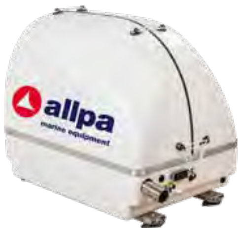
Paguro 4 SY Item Code G04100 Continuous electric power DIN @ 50Hz 4kVA – 3.5kW Weight (incl. soundproof hood): 83kg Dims. 636x433x547mm (lxwxh)
