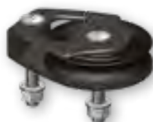
Item Code 5400611 Foot Block Weight = 0.13kg 2 x Ø6mm screws SWL = 800kg
