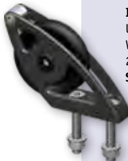
Item Code 5400616 Vertical Fix Weight = 0.14kg 2 x Ø6mm screws SWL = 800kg
