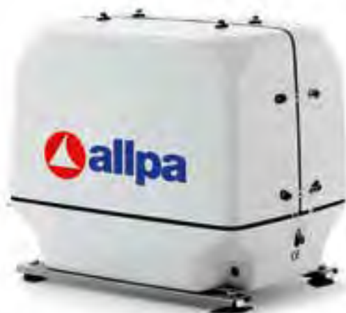
Paguro 9000 V Item Code G09100/V Continuous electric power DIN @ 50Hz 9kVA – 8kW Weight (incl. soundproof hood): 150kg + 15kg (Inverter) Dims. 686x487x615mm (lxwxh) Generator Dims. 250x220x330mm (lxwxh) Inverter
