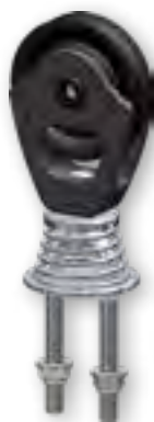
Item Code 5400613 BLOCK U-BOLT Weight = 0.22kg 2x Ø6mm screws SWL = 800kg
