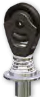
Item Code 5400715 BLOCK SCREWED Weight = 0.75kg 4x Ø6mm screws SWL = 1300kg
