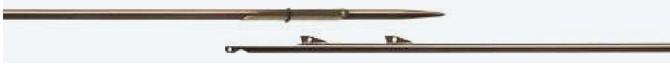
17-4PH steel rod with 2 fins, machined from solid CNC and laser welded. Bottom-mounted 1.2mm fin with a welded pin; tricuspid point.
