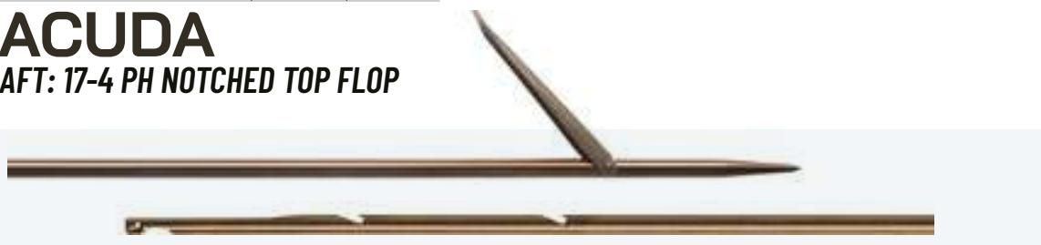
17-4PH steel rod with coupling notches, machined from solid CNC and laser welded. 0.8 mm lower fin with a welded pin; tricuspid point.
